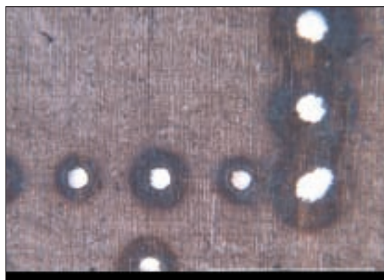
Fig. 4 — Inconel plate with seven machined holes is shown with a low magnification overview. The image was collected using simultaneous transmitted and reflected illumination.
